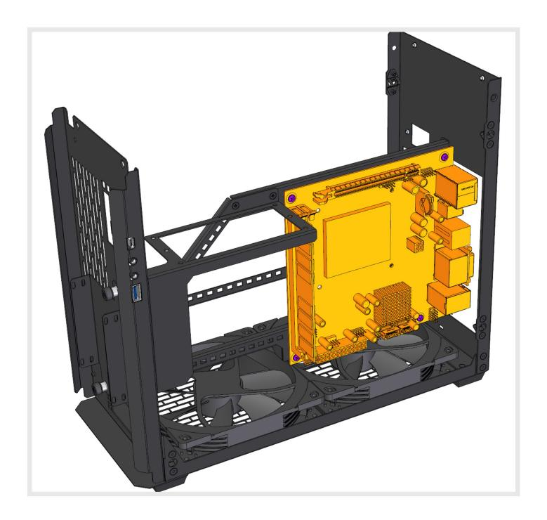
The motherboard is mounted with 4x M3.5 TRUSS HEAD screws.
