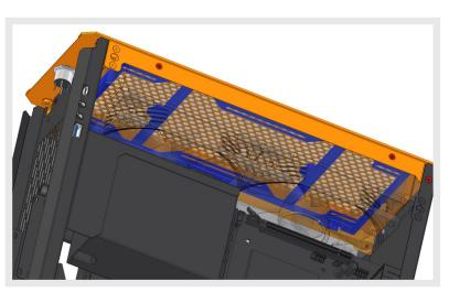
THE RADIATOR MOUNT BRACKET MUST HAVE THE ROUND KNUBS / HANDLE MOUNTS POINTING TO FRONT OF THE CASE.
