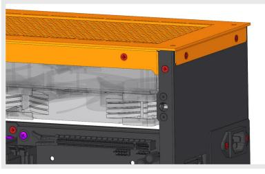
FLANGE ON REAR EDGE OF TOP MUST GO ON THE OUTSIDE OF THE REAR OF THE CASE.
