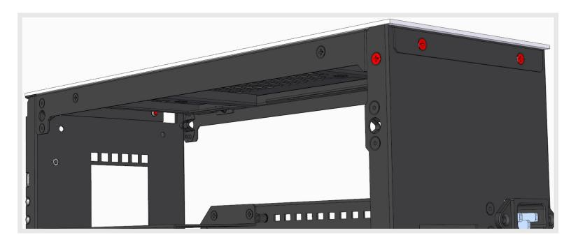
REASSEMBLY NOTE: When putting the top panel back on the case it is receommended to position the tabs on the rear corners first, then place the rear flange onto the outside of the frame. This will position the front flange
