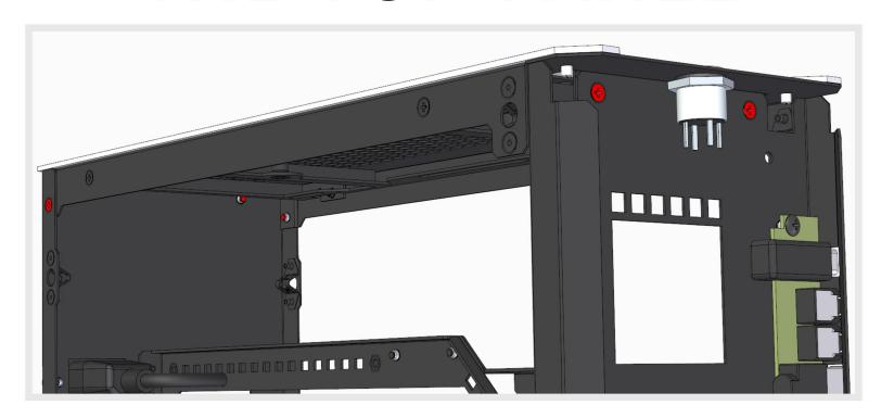
The top panel on the SM570 / SM580 is held on via 6x M3 flat head screws.
