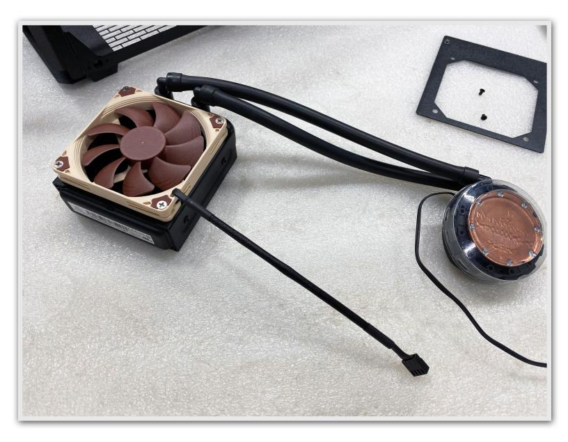
NOTE: Sliger does NOT include the screws for attaching the fan to the radiator. We recommend 4x .750" long 6-32 Phillips #2 flat head screws.
